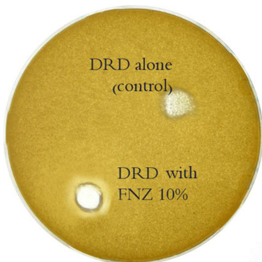
Fig. 4 Demonstrating the zone of inhibition of the Candida albicans growth around the well that contained the DRD with 10% fluconazole antifungal drug. Note the absence of an inhibition zone around the well that contained the control, i.e., the PMMA alone
